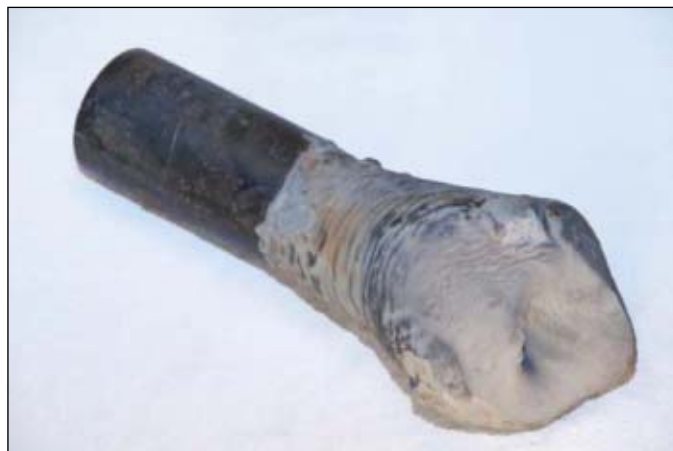
This nahcolite ( \text{NaHCO}_3 ) accumulation due to evaporation is on the end of a half-muleshoe that was at 3,000 ft in a San Juan basin gas well (Fig. 6).
