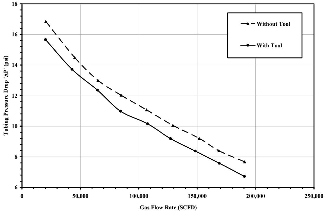
Fig. 5 – Effect of Number of Inlets on the Tubing Pressure Loss ( $P_{BH} \approx 20-21$  psig)
