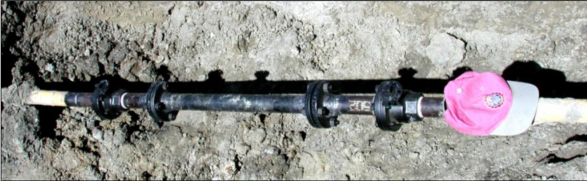
Figure 12 - RMOTC flanged flowline section to test for paraffin deposition. (ref. 12)
