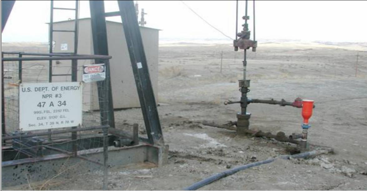
Figure 11 - Photo of the rod pumped 47-A-34 well with standard SX tool. (Ref. 12)
