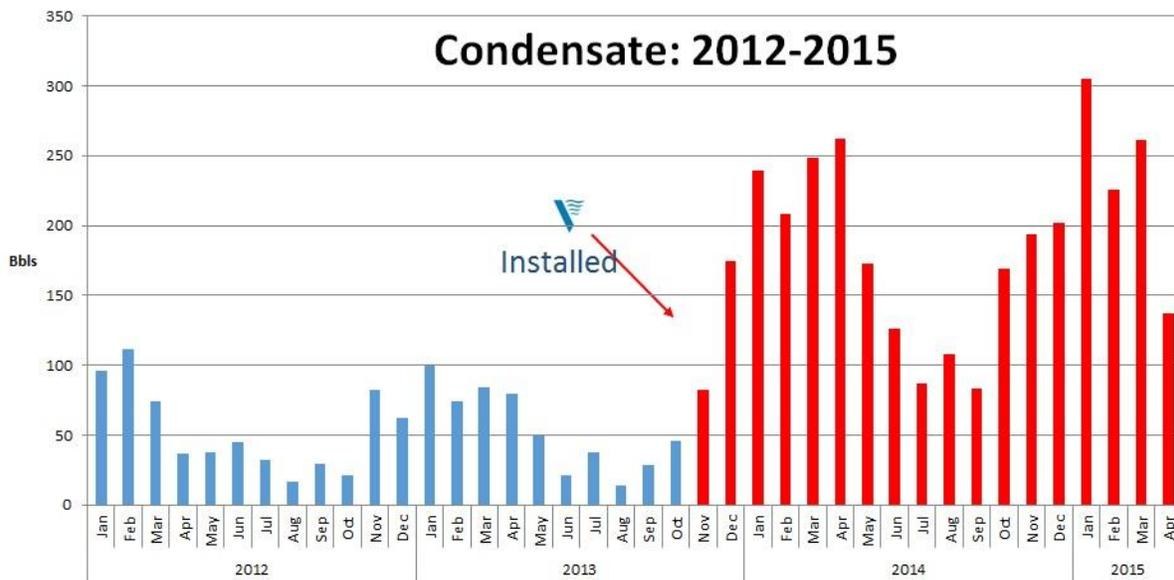
In addition to the 20 months with Vortex vs. the 20 months without Vortex data comparison, Vortex Tools compared a full calendar year with Vortex to the last full year without. As the tools were installed in October 2013, 2012 (12 months with no Vortex) was compared to 2014 (12 months with Vortex):
