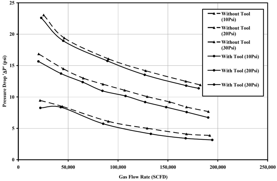
Fig. 7 – Effect of Pressure on the Tubing Pressure Drop
