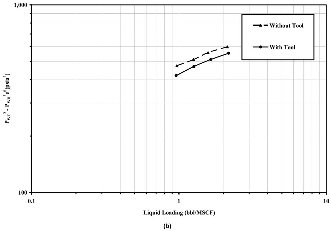
Fig. 9 - Pressure Loss at Different Liquid Loadings at
