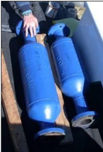
Figure 18. In-line VF units delivered for testing at 76-MX-3. The in-line design allows for simplified installations. The units were labeled #1 (long unit) and #2 (short unit).
