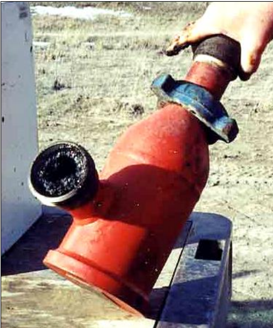
Figure 13. Paraffin buildup at the VF unit inlet at the end of testing on 1/13/04. Blockage resulted after the well was treated for downhole buildup.
