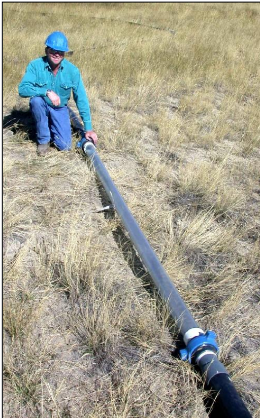
Figure 20. A ten-foot clear plexiglas line at the wellhead of 76-MX-3. Entrained water would form a spiral pattern on the interior wall. The long in-line VF unit gave the most efficient spiral pattern of the units tested. Stripper Well Consortium members viewed this flow character during a visit in September 2003.
