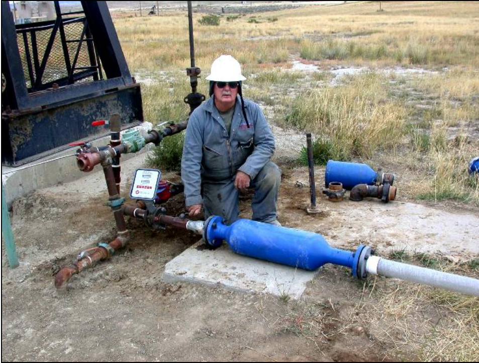
Figure 19. Long in-line VF unit #1 installed at well 76-MX-3. Note Halliburton flow meter.
