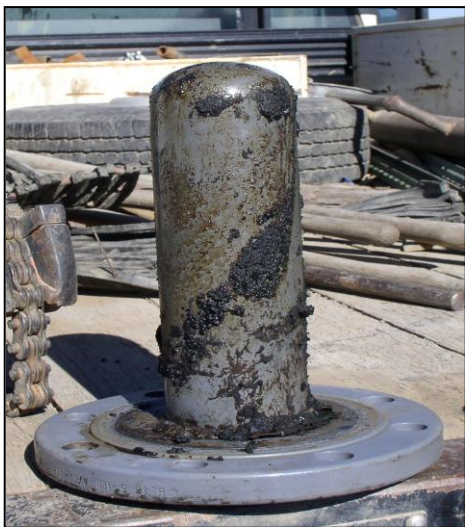
Figure 10. Dissassembled flanged VF unit after 30 days of operation
